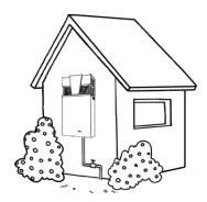
This water heater must be installed vertically upright with the water and gas connections on the underside, pointing toward the ground. The back of the water heater can be either against a wall or supported by a frame.
